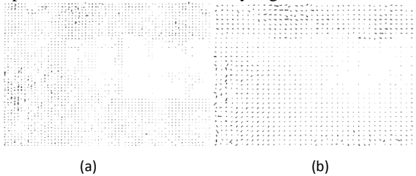
Fig 3: Optical flow of Yosemite with clouds using a) HomSchunk (Global Flow) method b) Lucas-Kanade (Local
